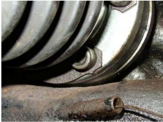
Once done, make sure that the CV joints can't foul the horns when there's gearbox movement on the mounts. I increased the gap slightly between the CV joint and the frame horn after this pic was taken.
