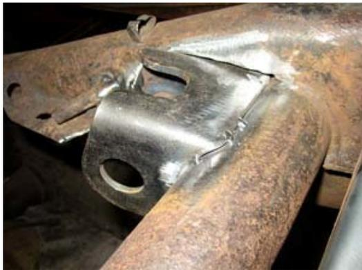
Once they can be fitted up in place, ensure the area is thoroughly cleaned and free from rust and dirt so it can be welded. Then tack the brackets in place. Only enough to hold it in place though as you may need to adjust them if they are not perfectly aligned. This is what you should end up with:
