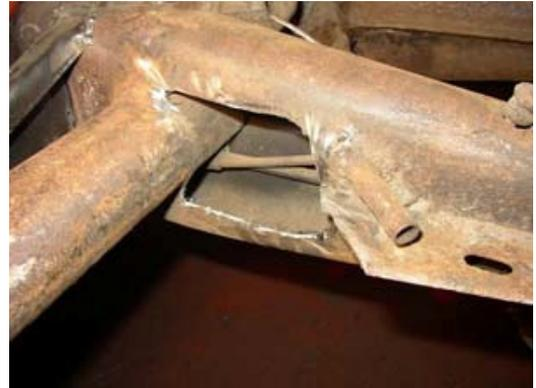
You should end up with a hole in the side of each of the frame horns where the IRS brackets recess into them. The depth of the hole shown below is about an inch too low as I got the jig in the wrong position when first marking it out - oops! As such it will be filled with fresh metal when it comes to fitting the brackets permanently.
