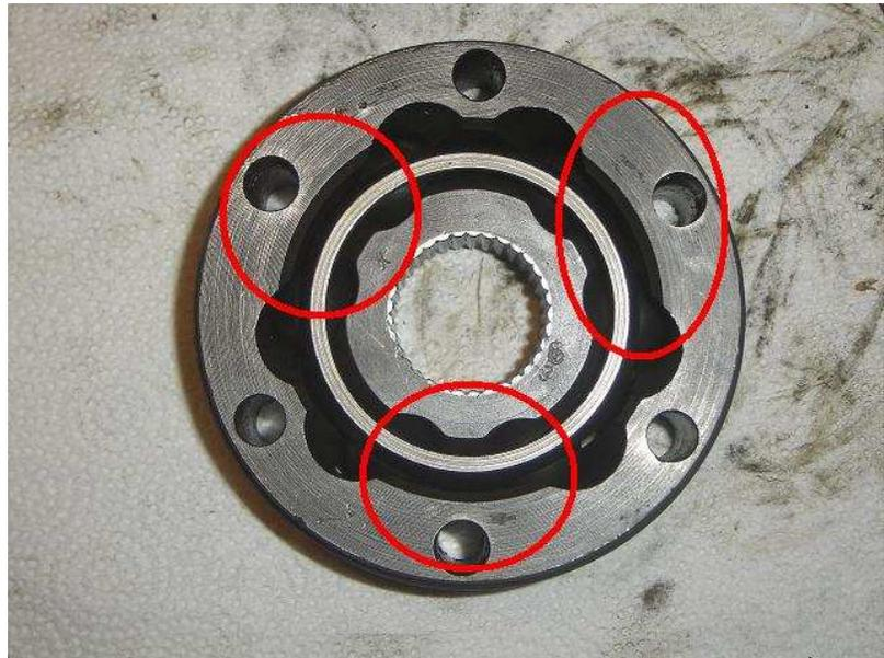
I find it easier to grease the joints before installing them on the axle. But your mileage may vary. Get out your grease. If you bought new CV boot kits, they should come with tubes of grease for you to use. If not, get your grease from the parts store. Make sure your grease is intended for use in CV joints, it will usually say that on the packaging. It will also say it's an "extreme pressure" grease.
