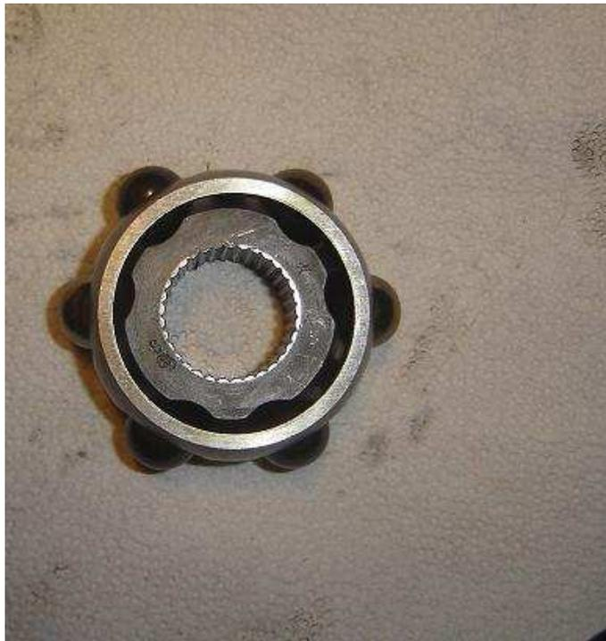
If your CV looks like the one shown then it is wrong. Notice the points that are circled. The narrow point on the inner race should not line up with the narrow point on the outer race. The narrow point on the inner race should line up to the broad section of the outer race. Notice the picture shown on the right, this is wrong.
