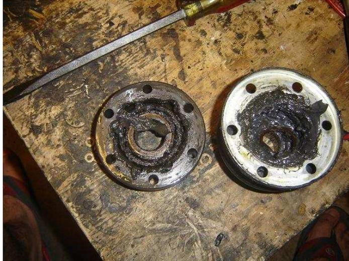
First you want to disassemble the joints. Push the hub out like you are trying to make the hub perpendicular with the outer race. This will cause some of the ball bearings to fall out, which will make the rest easier to get out. Then the cage and hub will come out of the outer race, and then you can twist the hub out of the cage.
